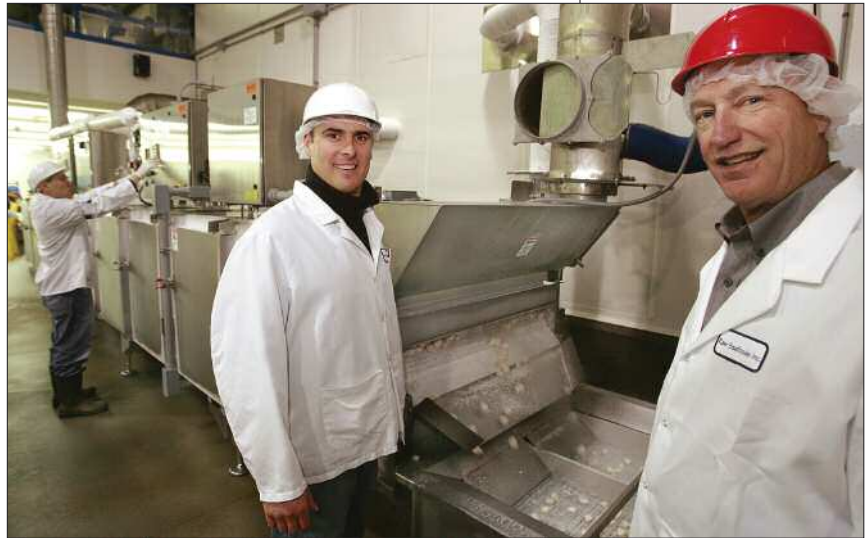
Individually quick-frozen scallops tumble off the conveyer belt of the Praxair ColdFront ™ ultra performance flighted tunnel freezer at the Raw Seafoods plant in Fall River, Mass. Pictured alongside the freezer are Raw Seafoods President Jason Hutchens, left, and Praxair’s Frank Martin.
