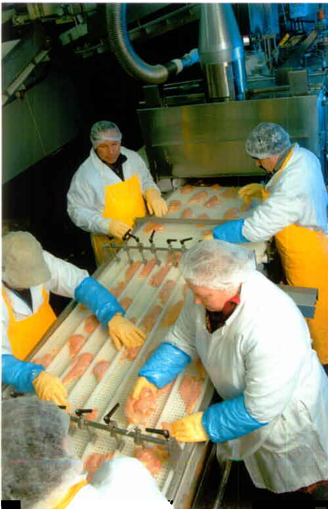
Whole chicken breasts pass through Praxair's immersion freezer before moving on to a ColdFront spiral freezer.
